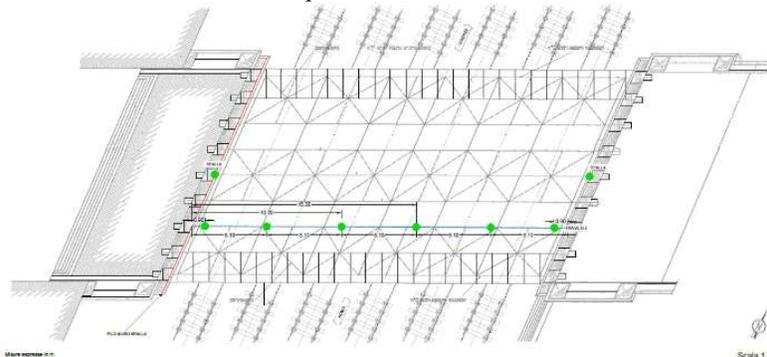
Figure 10 inclinometers positions
