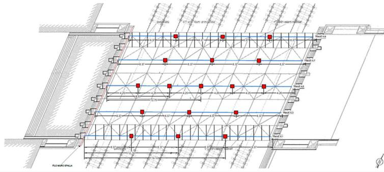
Figure 9 accelerometers position
