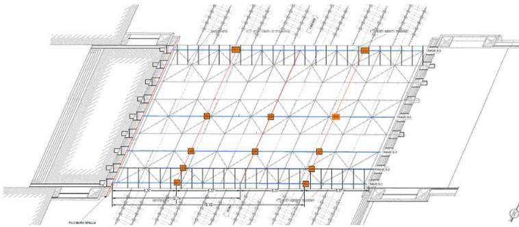
Figure 11 strain gauges positions
