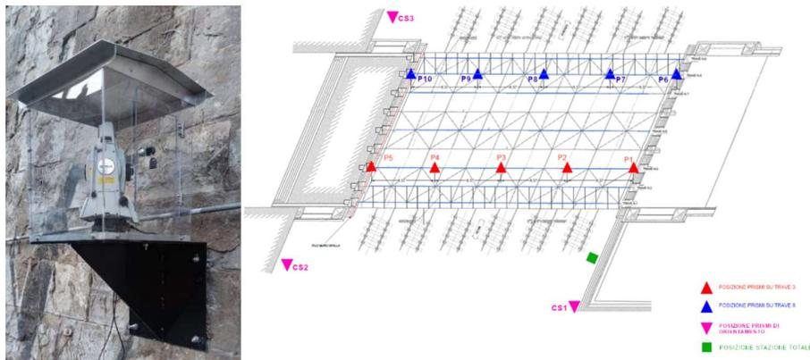
Figure 12 to the left automated total station, to the right prisms, cornerstones and total station locations
