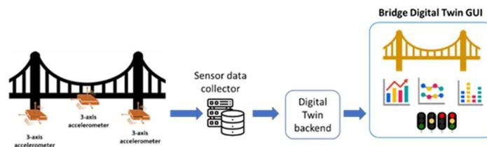
Figure 1 Conceptual architecture of the monitoring system.
